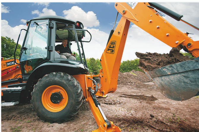
Available as an option on JCB 3CX and 4CX backhoe-loader models, the Easycontrol seat-mounted servo control system improves backhoe speed by changing from a flow-sharing valve block to a full-flow hydraulic system.
