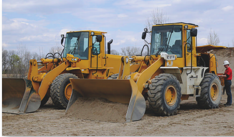
Identical 190- to 200-horsepower wheel loaders were powered by 6.7-liter QSB engines – one certified to Tier 3 emissions limits and the other performing to Tier 4 limits. The engines were specified with the same power output, peak torque and rated speed.
